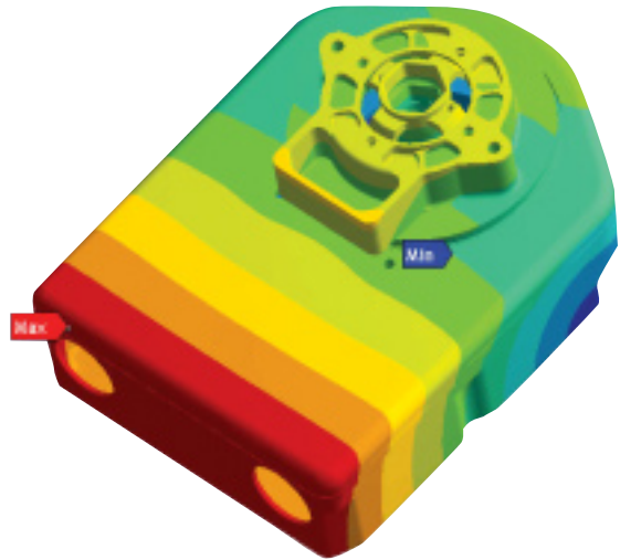
Deformation of the M-360 unit under extreme loading conditions, represented by the FEA results shown here
