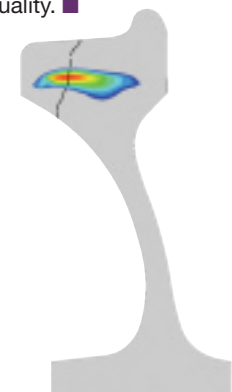
Vertical split rim and contours showing the residual tensile stress
