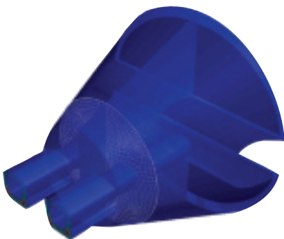
Fluid model extracted from solid CAD model
