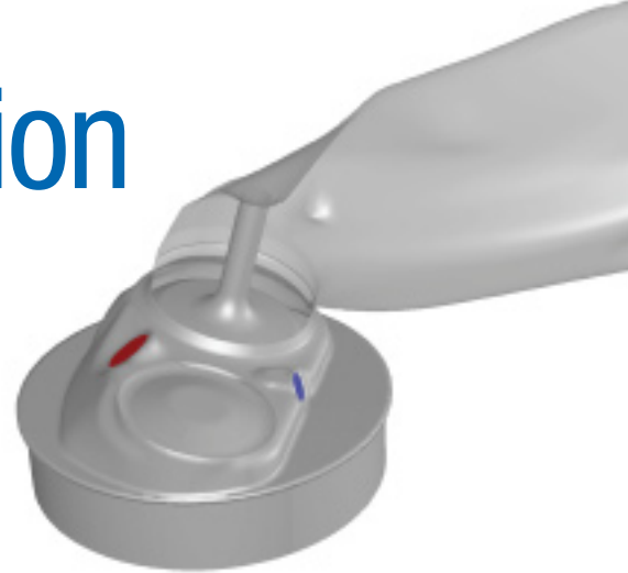
The geometry of the engine: the injector is located near the valves at the end of the engine cylinder as represented by the blue dot, while the spark plug is on the opposite side of the injector, located 3 mm inside the red dot.
